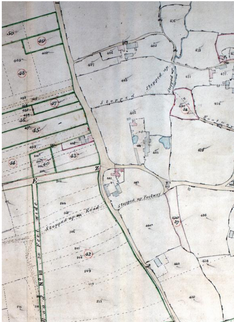
Fig. 5.5 One of the important changes affecting the landscape was brought about by the rationalisation of the road network. Before enclosure the road system had grown organically. The result was many routes that were convenient but not essential. The extract taken from the enclosure map of Charlton shows some of the steps taken by the commissioners as they closed old routes and created new ones.
